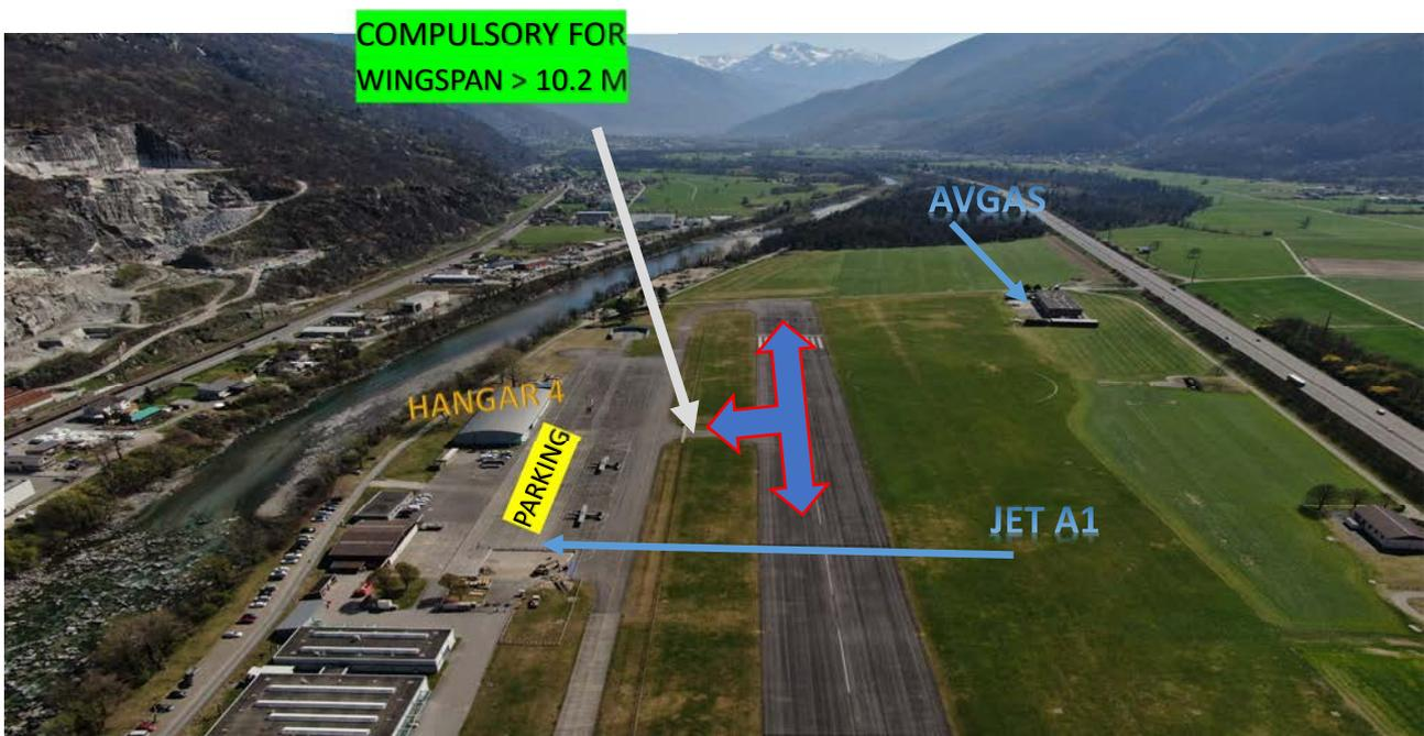
Aircrafts with a wingspan **> then 10.2 up to 15 m** need to enter or exit the runway via the gate located in front of Hangar 4, see picture above.
