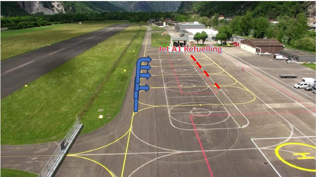
Despite as indicated in the old charts and on ground aircrafts must be parked facing east as shown in the figure above by the blue arrows.
